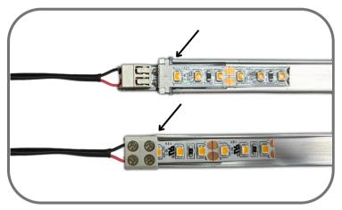
**Step 9:** Remove adhesive backing from LED Strip and connectors. Carefully align connector with edge of aluminum channel and adhere along the center. For Tiger Paws, the black latch will be placed on the edge of the aluminum; for iDea Series Connectors, the base of the connector will be placed at the edge of the aluminum.
