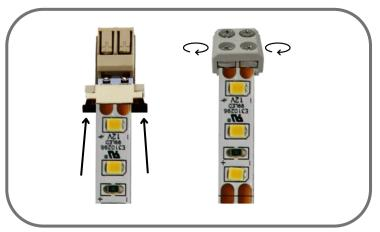
**Step 6:** If using a Tiger Paw, insert LED flex between black latch and bride connector, then slide latch closed. If using the iDea Series Connector, insert flex into connector and tighten screws.
