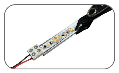
**Step 10:** Use dikes to cut aluminum to length as close as possible to the end of the LED strip. Snip each raised edge, and bend aluminum back and forth until fully separated.
