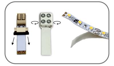
Step 4: Prepare to attach Tiger Paw or iDea Series Connector by peeling back adhesive lining from LED strip, and pulling open black sliding latch or loosen input screws.
