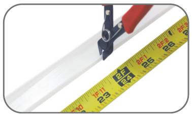
**Step 11:** Measure and cut plastic lens to length. For easiest cut, use dikes to snip each edge, then gently bend plastic back and forth until fully separated.
