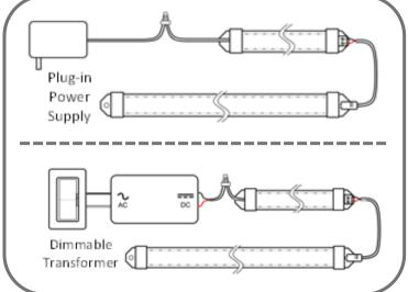
**Step 16:** Follow corresponding instructions to incorporate switches, dimmers, power supplies and transformers for a complete LED system.
