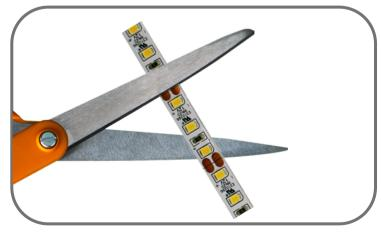
Step 3: Use scissors to cut along copper pads located closest to subtracted measurement without going over.
