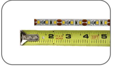
Step 2: Determine length of LED strip by taking total available space and subtracting 1.5" for each connector needed If using a connector on one side, subtract 1.5" total; a connector on both sides, subtract 3" total.
