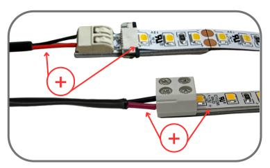
**Step 7:** Identify the polarity marked along the stripthis will determine polarity of wiring. *Positive wire will align with positive side of LED flex strip.*
