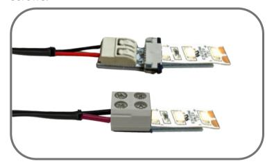
**Step 8:** Use power supply to test strip functionality. If lights do not turn on, double-check that polarities are properly matched. Repeat steps 4-7 to add connectors to opposite sides of flex.
