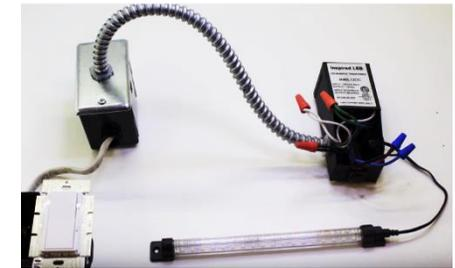
**6** Connect to LEDs with standard plug-in or screw terminal, mount transformer in well-ventilated area, turn on main power, and test switch
