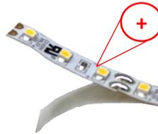
**4** Insert strip into the gap between black sliding latch and beige bridge piece, matching polarity of strip to (+) signs on Tiger Paw<sup>®</sup> board.
