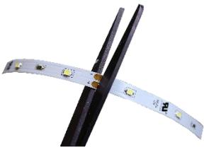
**2** Take hold of black sliding latch and pull outward to open, taking note of (+) polarity marked on board.
