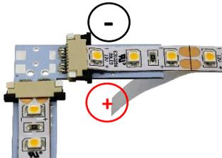
**7** LED strips should be centered and fully inserted before sliding black latches firmly closed.
