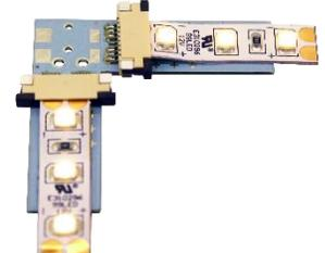
**Troubleshooting:** If LEDs are flickering, double check connection to be sure flex is fully inserted and secured, if no lights turn on check to be sure polarities are properly matched. **Marked polarities on Tiger Paw may be ignored as needed to change direction so long as polarity matches from strip to strip.**
