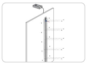
**Step 7:** Secure drywall reveal in place using sheetrock screws every 12"–18". Excess stud mount screws from step 5 may be removed if desired. Tape wire drop in place to prevent loss or damage before proceeding.
