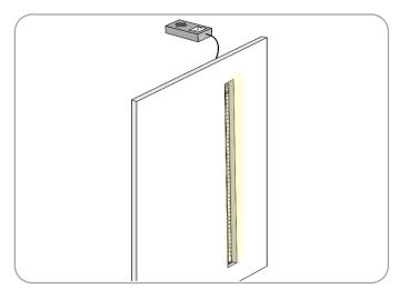
Step 18: After all LED strips have been installed, turn on power to test full system. Ensure that all diodes turn on and that they respond to dimming (if applicable). Once satisfied, turn off LEDs to complete install.
