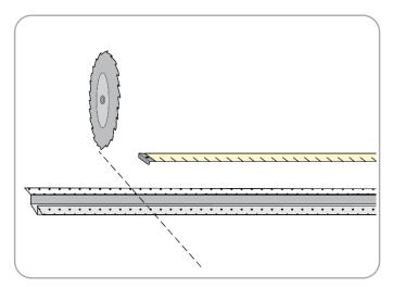
**Step 1:** Measure and mark desired length of wall reveal. Cut using table saw and appropriate blade designated for plastic or aluminum (depending on selected material).
