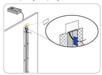
**Step 8:** Position mud caps on top and bottom edge of aluminum with **narrow** lip facing outward. Ensure wire drop notch is completely covered by mud cap and secure with construction adhesive.
