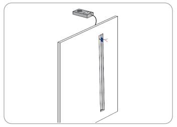
**Step 11:** When mud and/or paint is dry, remove painters tape from wall reveal. Ensure that wire drop is still in place, and that the space is free of mud or debris.
