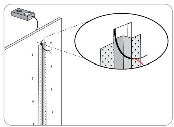
**Step 6:** Insert wall reveal into hole. Cut a small notch out of the top no taller than 1" and no wider than 1.5" to ensure it will be covered by mud-cap. Carefully pull wire drop through this opening.
