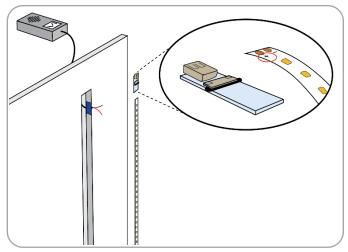
**Step 13:** Prepare LED strip to be inserted into Microlock Tiger Paw® by identifying polarity marked along the strip with +/- symbols. Positive polarity will be matched to your wire drop in step 16.
