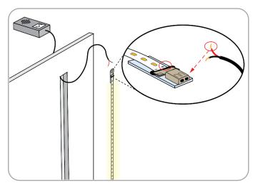
**Step 16:** Strip back ends of wire drop about ½". Match the positive side of cable to positive side of LED strip, then insert both polarities into beige micro-lock. **Ensure that lights are functioning** before moving on to next step.
