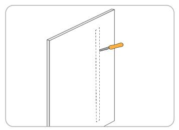
**Step 3:** Use oscillating saw or jab saw to cut away the marked drywall. Clear away as much debris as possible from inside the wall.
