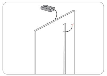
**Step 4:** Use in-wall rated **solid gauge** cable to create wire drops from Class 2 12V or 24V DC power supply to desired locations, leaving at least a 12" lead. Test power supply and wire drops to ensure functionality.
