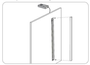
Step 20: Once all steps have been completed and double checked, carefully align lens with the top or bottom edge of wall reveal and press firmly into place. If experiencing difficulty, be sure no mud or debris is blocking the reveal.
