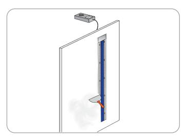
**Step 9:** Use painter's tape to protect the interior of the wall reveal. Then, follow brand or industry instructions to apply joint tape and drywall mud over edges and mud caps. Spread evenly from the mud ridges over the wings.
