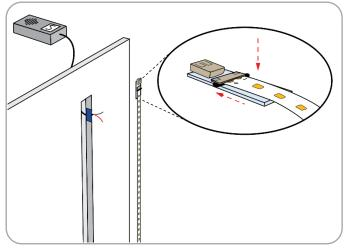
**Step 15:** Slide the black Tiger Paw<sup>®</sup> latch closed and firmly press LED strip adhesive onto board to secure connection.
