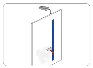
**Step 10:** For best results, apply at least four coats of mud for even blending, waiting for each layer to dry before adding another. Finish drywall with plaster, texture, and paint before proceeding to next step.
