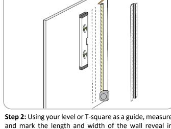
**Step 2:** Using your level or T-square as a guide, measure and mark the length and width of the wall reveal in desired location on drywall. Final cut-out should measure 3/4" wide.
