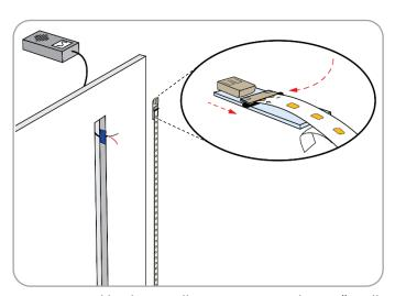
**Step 14:** Peel back LED adhesive covering about 1". Pull open the black sliding latch on the Tiger Paw® and insert flex strip just below the beige bridge piece.
