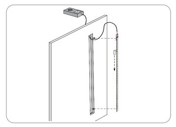
Step 17: Remove adhesive backing from Micro-lock Tiger Paw® and from LED strip, then carefully adhere along the inside of channel. Strip should be aligned as straight as possible for even light distribution.
