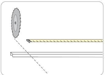
Step 19: Measure length of exposed wall reveal to determine the required size of lens pieces. Mark lenses and use a table saw to cut to length. Do not use handheld dikes or clippers as this may crack lens material.
