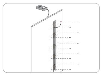
**Step 5:** Identify studs behind hole to which wall reveal can be mounted. If necessary, create studs every 12"-18" using wood planks no less than ¾" thick. Mount using countersink sheetrock screws.
