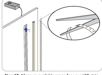
**Step 12:** Measure available space for your LED strip. Cut strip to length on **copper pads only**. If selecting between two cut points, use the shorter length.
